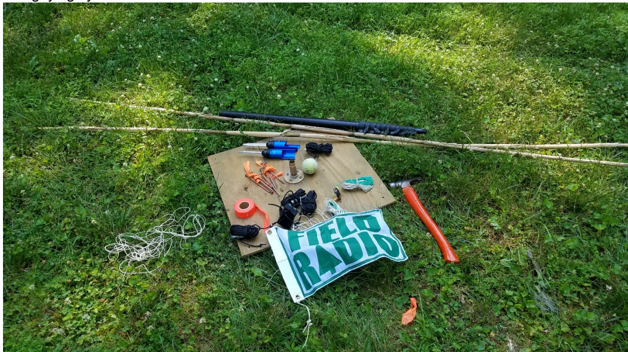
Figure 1 Base plate made of plywood with floor flange for Buddipole 16 ft mast
