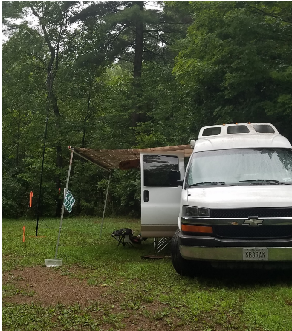
Figure 3 Antenna position too close to the RV.
