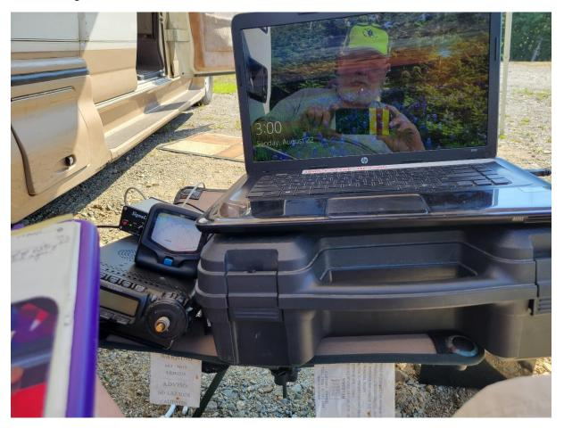
My station was a Yaesu FT857 to a SignaLink USB to a Radio Shack SWR meter to a MFJ 1620 Hamstick or a home brew 20- or 40-meter dipole in an inverted vee aimed roughly southwest. I used a EZ Hang slingshot with a fishing reel and a lead weight to shoot the line over a sturdy branch after about 3 tries. It held all weekend. The RigExpert AA-230 Antenna and Cable Analyzer was handy to check that antenna connections and cables were working.
