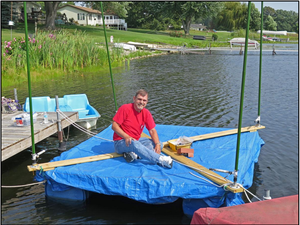
KC9UR setting up the 20M Floating 4-Square swim-raft-mounted antenna
