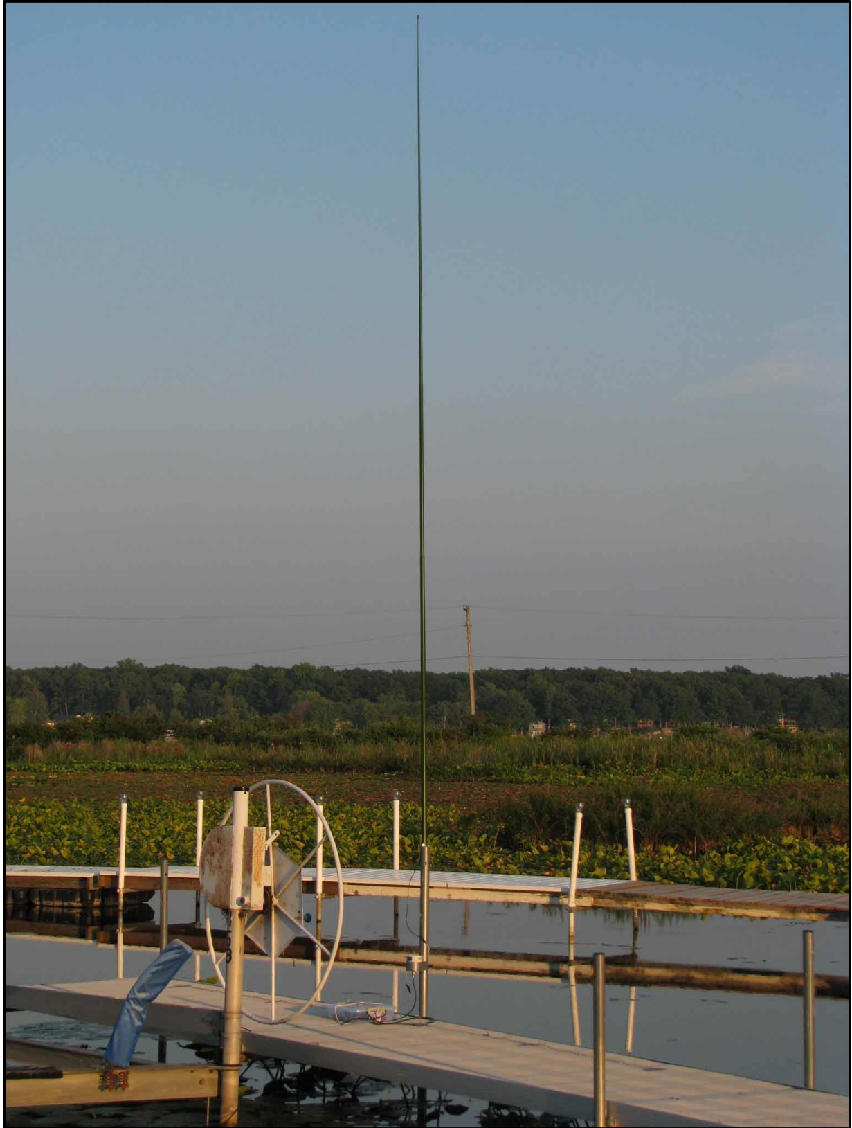
Figure 3 - 18 ft vertical antenna mounted to the pier
